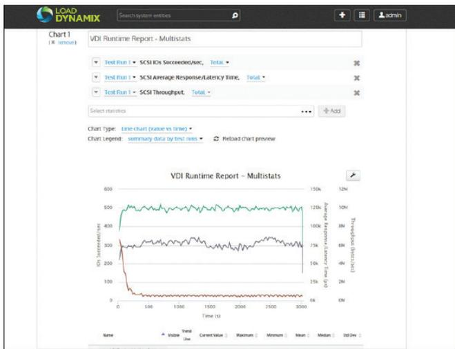
Figure 9: Multi-statistics report, showing IOPS, latency, and throughput on a single graph
